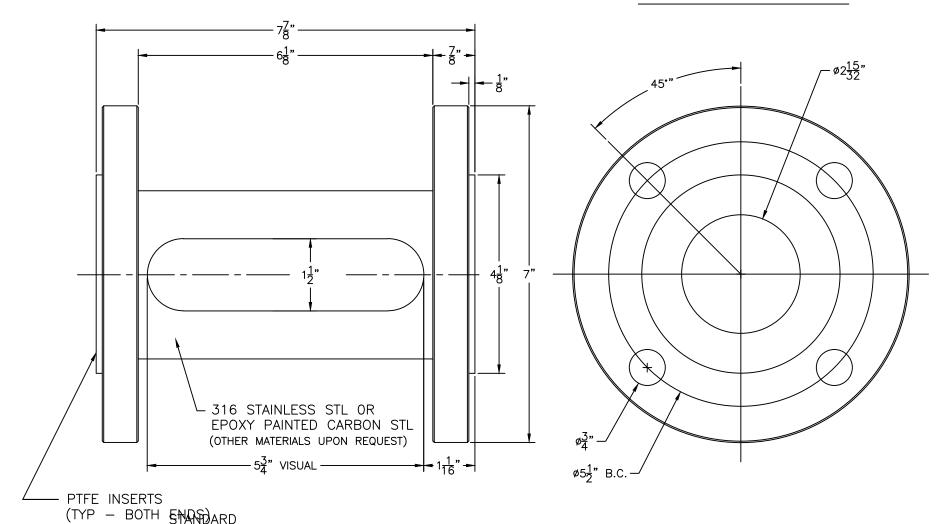
O-RING SEALS [NOT SHOWN] STANDARD: BUNA-N, EPDM, FLUROELASTOMER [FKM]
